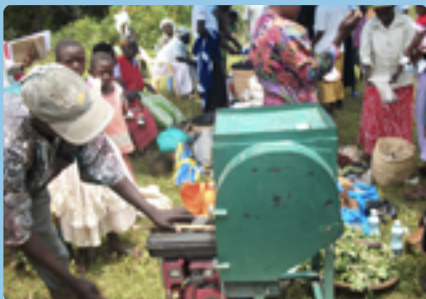
Figure 3: This is a manual thresher for vegetables, cassava, napier grass and any other farm produce into smaller particles as part of the value adding process
